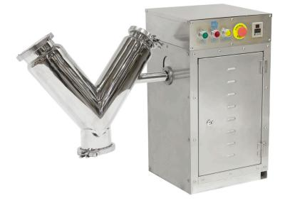
The VM<sup>®</sup> Lab Mixer Range consists of powder mixing machines designed for combining dry powdered materials to produce a homogeneous mixture of multiple powders together. Coming in sizes of 2 L, 10 L and 15 L, the VM<sup>®</sup> Lab Mixer Range is the perfect mixing device for laboratories and R&D departments.
