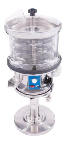
The TDD 1<sup>™</sup> Tablet De-Duster removes excess powder from tablets using compressed air and a vacuum. The tablets simultaneously move around a five-layer agitation plate, which loosens any residual dust. With the ability to clean more than half a million tablets an hour, this machine can also be used in conjunction with a tablet press so that the tablets pour into the de-duster right after being pressed.
