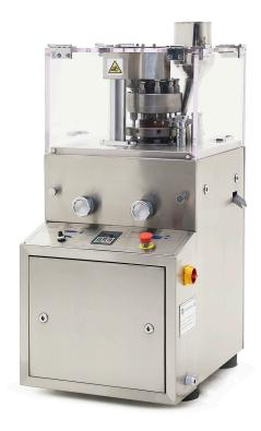
The RTP 9® is a sophisticated rotary tablet press that allows users to produce large volumes of top quality tablets rapidly and efficiently. Among the RTP 9®'s advanced features are a digital interface and convenient control console. Together, these make it easy for the operator to manage the machine without having to make time-consuming manual adjustments to bolts and screws.
