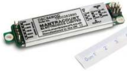
DSC Card version available the strain gauge data converter to RS232. Modbus, CAN, RS885
